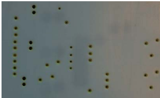
Incomplete cleaning of adhesives due to inability to penetrate apertures
